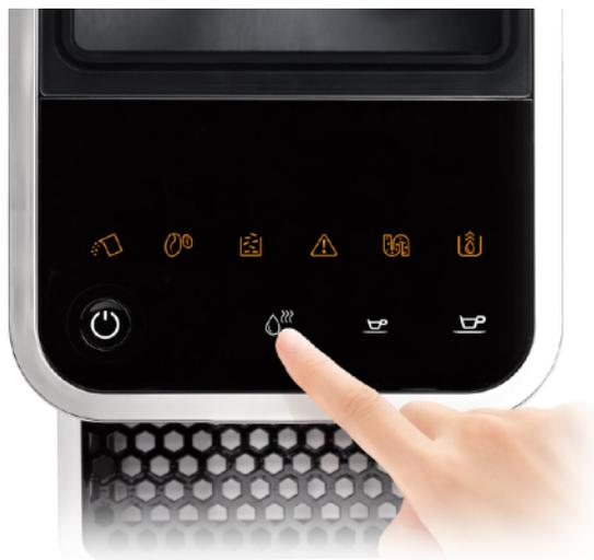
The controls are situated on top of the machine at the front and consist of a touch panel with a **Power** button on the left, a **Hot Water** button, an **espresso** button and a **lungo** button. The espresso and lungo extraction volumes can be programmed by holding the button and releasing when the desired output is achieved - thereafter just press once and voila.
